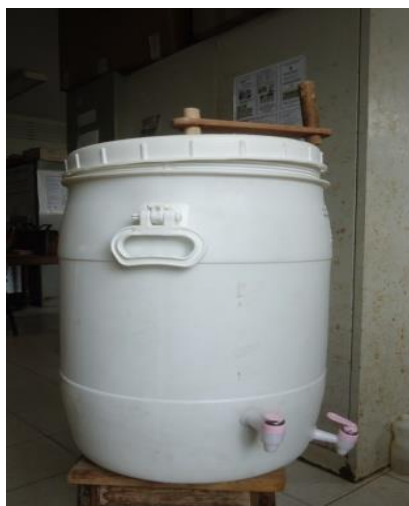
Fig. 1. Struvite reactor adapted from the Nepal model (Etter et al., 2011)
